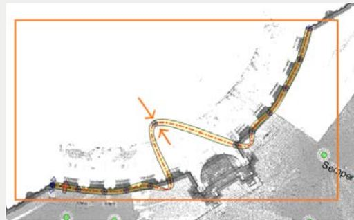
In the definition of the section view we can define the influence area of the point cloud. In one of the side views the height of the section can be edited by dragging the arrow up or down.
